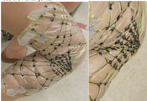
Figure 2. Recreation of Iberall's lines on a full-scale replica of a current subject, with Kevlar and epoxy garment overlaid on top. Yellow fibrous strands are Kevlar; black or white dots are epoxy sealant used to fuse the Kevlar joints.
