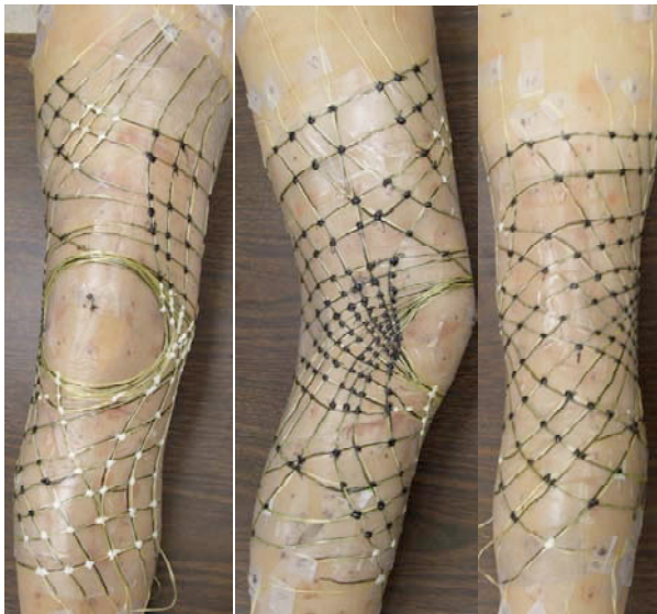
Figure 2. Recreation of Iberall's lines on a full-scale replica of a current subject, with Kevlar and epoxy garment overlaid on top. Yellow fibrous strands are Kevlar; black or white dots are epoxy sealant used to fuse the Kevlar joints.
