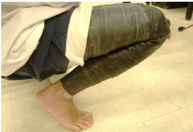
Figure 2. Subject demonstrating deep knee squat to a knee flexion angle of approximately 150°, significantly higher than the ~80° achieved in previous MCP leg garments [1].
